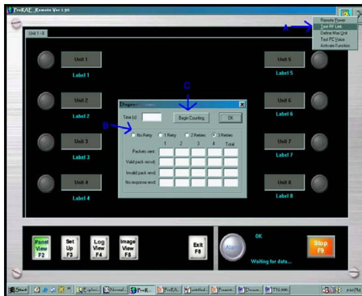
Figure 1. Advanced Tools>>Test RF Link. Select the Advanced Tools icon (A) and choose 'Test RF Link'. Choose the number of retries (B) and proceed to hit 'Begin' (C).
