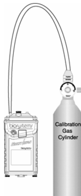
Figure 4.1 Bump Test and Span Calibration set up
